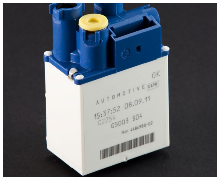
Contrasted marking on plastic without any additives
