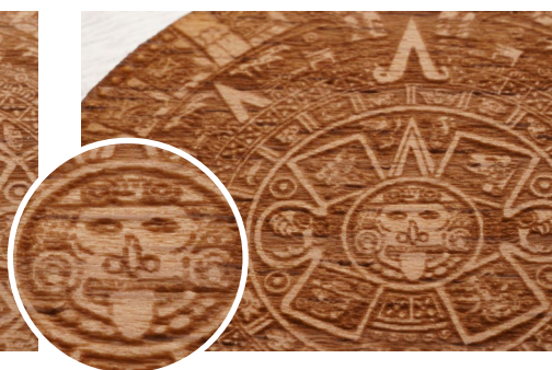
4.0" engraving A rough engraving that looks blurred
