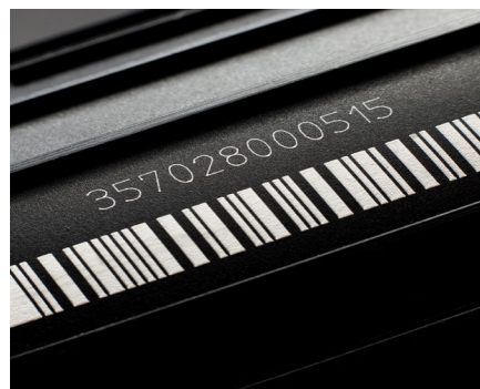
Contrasted marking on plastic
