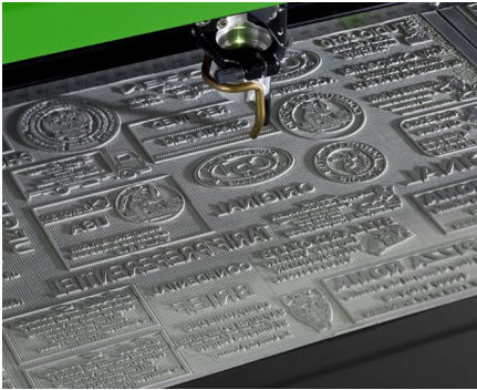
Engraving & laser cutting of custom ink stamps
