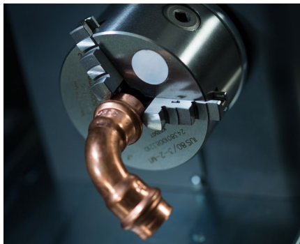
Rotary accessory for cylindrical parts marking
