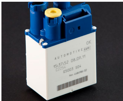
Contrasted marking on plastic without any additives
